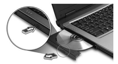
Insert a clip to the emergency eject hole to eject the optical drive tray when the computer is off.
